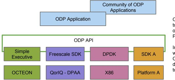
ODP demonstrated to run at negligible overhead on several Platform SDKs
