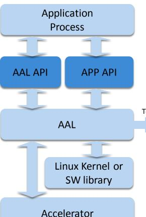
AAL API is for runtime accelerator (or virtual accelerator) detection, allocation, binding, initiation and access.
