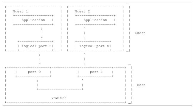
HOST 1(Physical port  $\rightarrow$  virtual switch  $\rightarrow$  VNF  $\rightarrow$  virtual switch  $\rightarrow$  Physical port)  $\rightarrow$  HOST 2(Physical port  $\rightarrow$  virtual switch  $\rightarrow$  VNF  $\rightarrow$  virtual switch  $\rightarrow$  Physical port)
