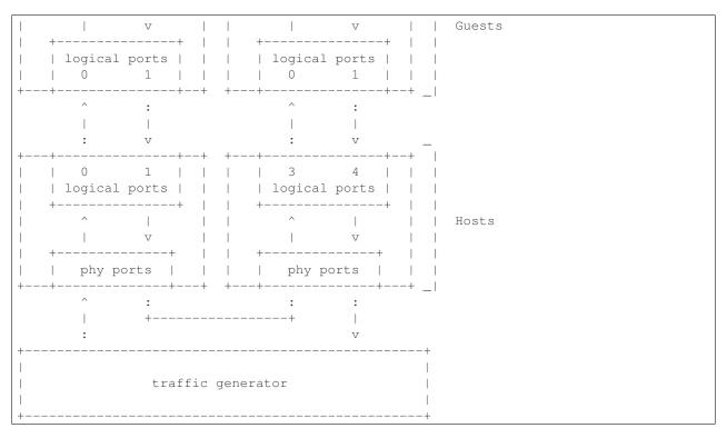
**Note:** For tests where the traffic generator and/or measurement receiver are implemented on VM and connected to the virtual switch through vNIC, the issues of shared resources and interactions between the measurement devices and the device under test must be considered.
